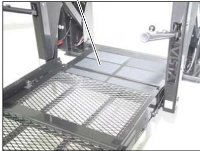
Fully-Unfolded (horizontal) Bridge Plate (bridging position)
